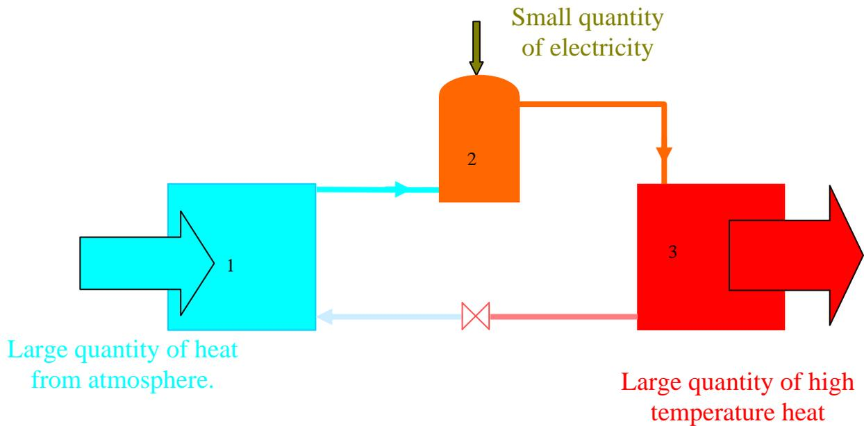
Energy is extracted from the air or from water condensing out of the air onto the evaporator.
